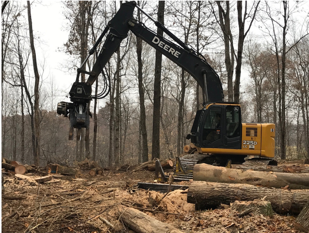
An excavator with a cut off saw attachment makes log processing safer and faster.
