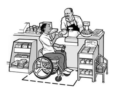
A lowered counter and clear floor space are critical components of an accessible service counter.
