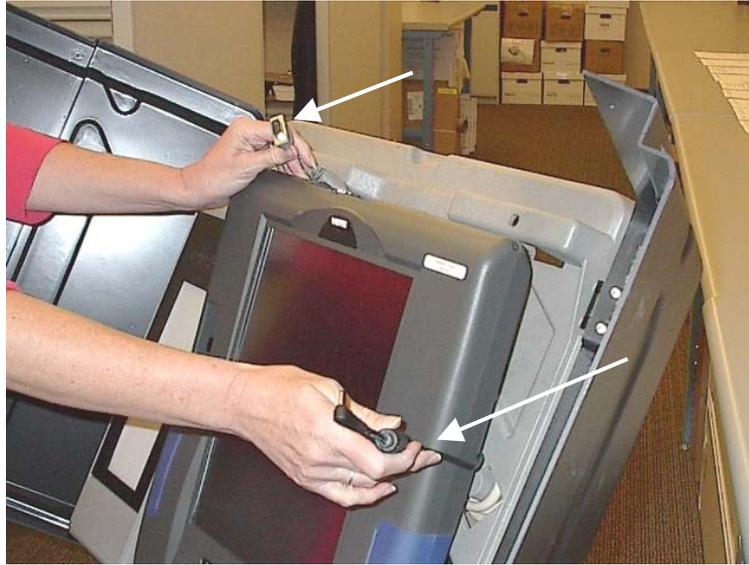
10. Attach the black cable to the top of the voting machine to connect the machine to the AC adapter.
