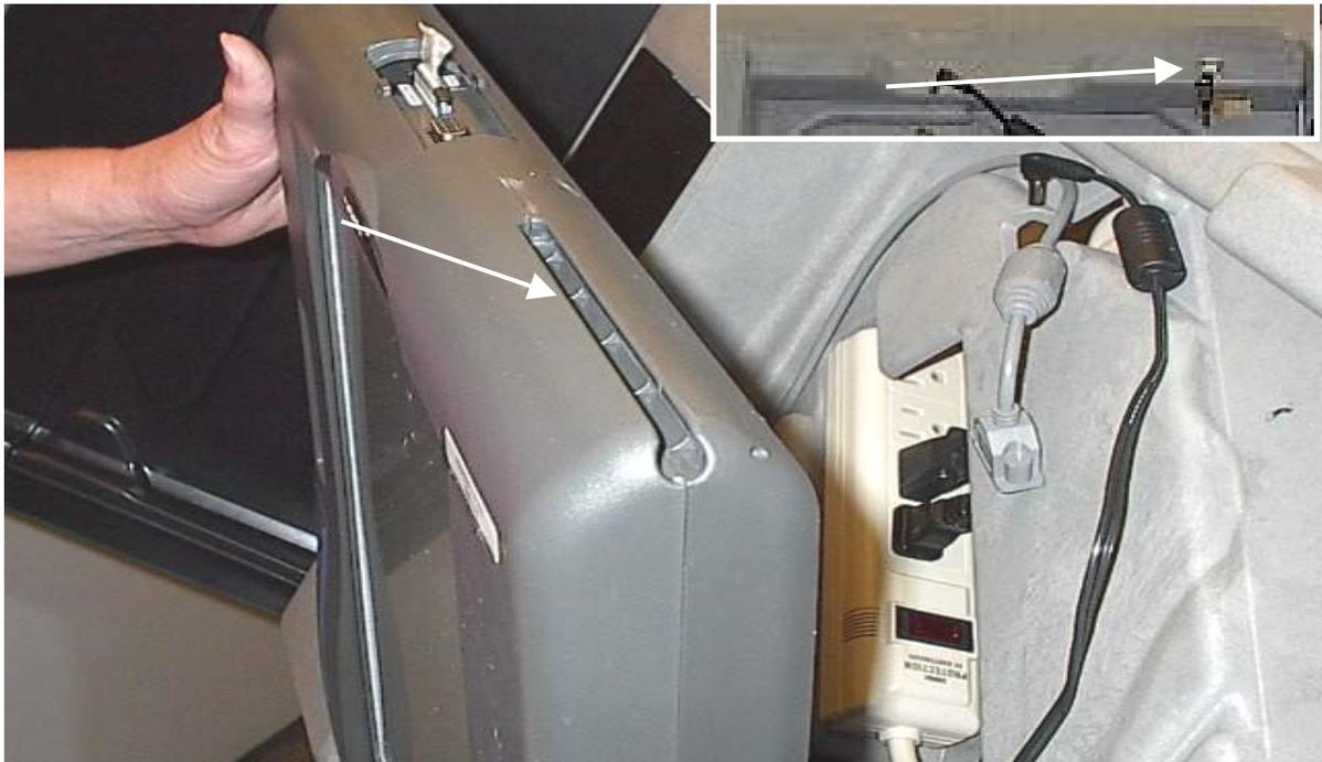
11. Lock the voting machine into the booth by turning the key to the right. The lock fits into the slot at the top of the iVotronic voting machine.
