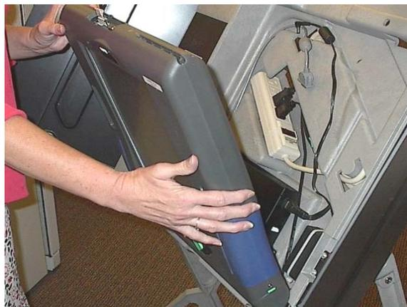
9. Attach the grey serial cable to the top of the iVotronic voting machine to connect the machine the printer (if one is included)
