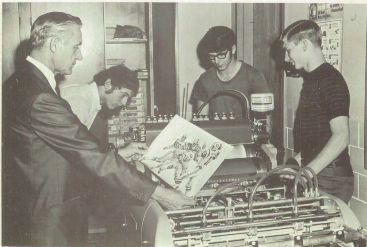
Mr. Bradfield is instructing his third hour printing class in the operation of the new off-set machine.
