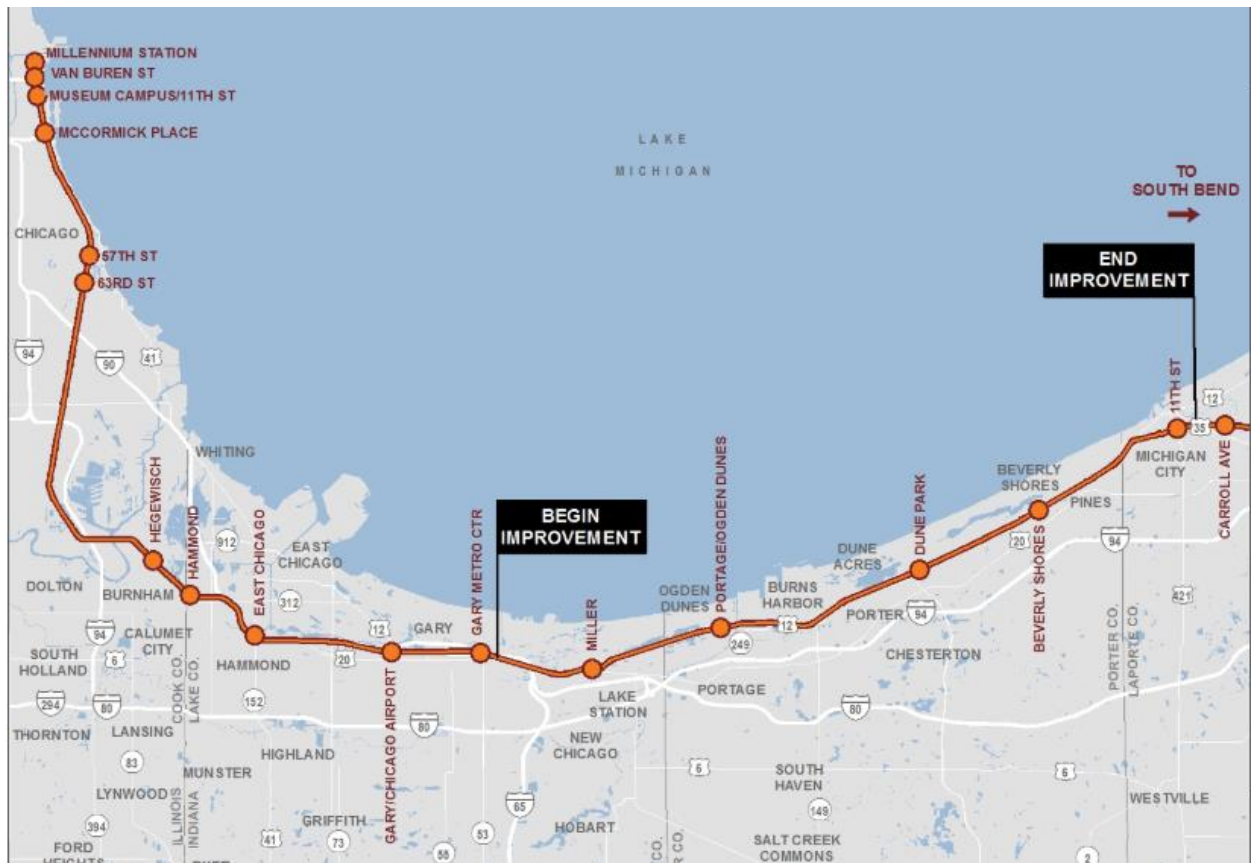
Double Track Northwest Indiana Project 25-mile second track between Gary and Michigan City
