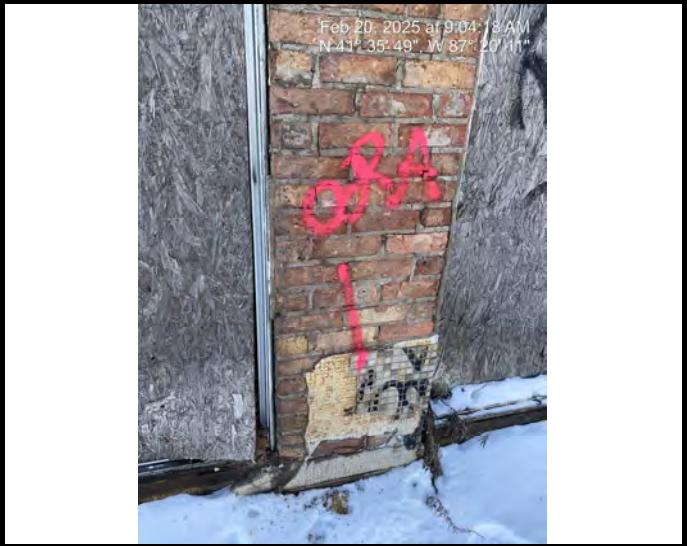
Sample # 8 Ceramic Tile - w/ Grout & Mortar, gray/white/yellow
