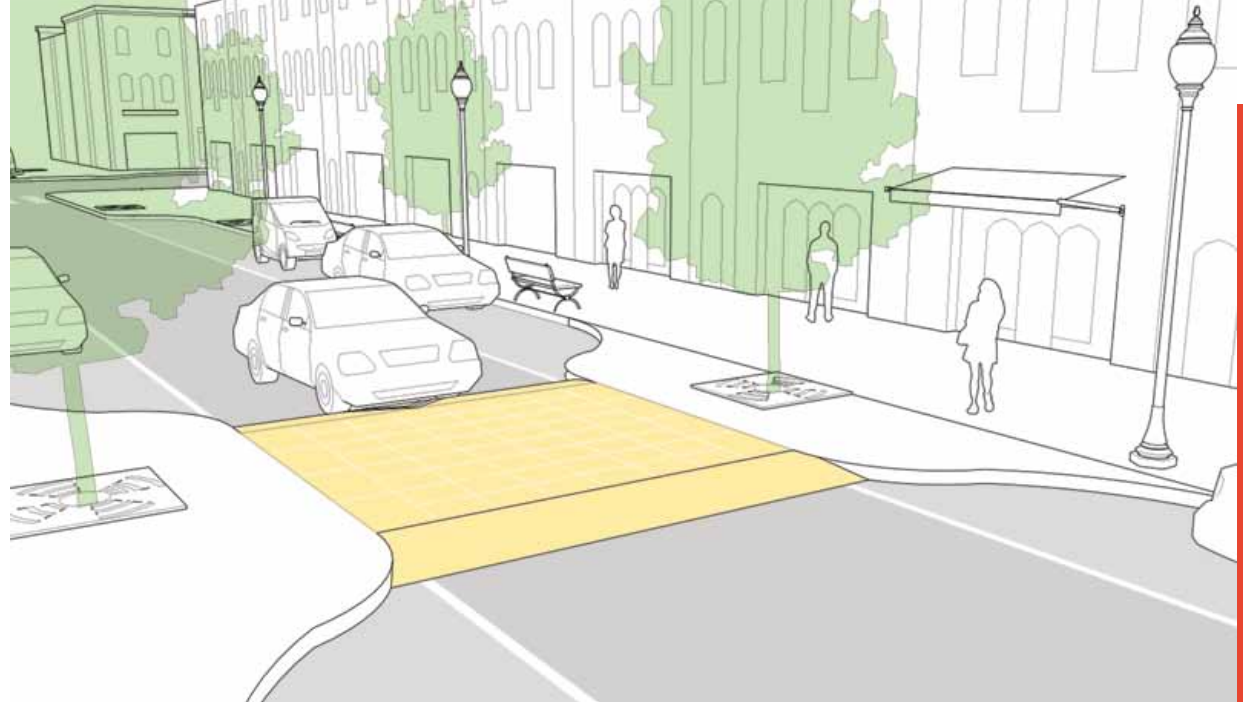
Speed Table at Mid-Block Crossing
