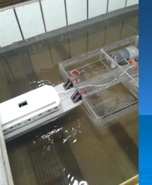
Simulated Barge Movements in Confined Channels / **Potential Fish** Entrapment
