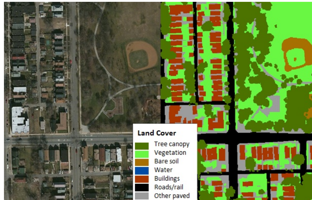
Fig. 1: Comparison of satellite image and land cover map. Seven types of gray and green infrastructure are in the land cover map.
