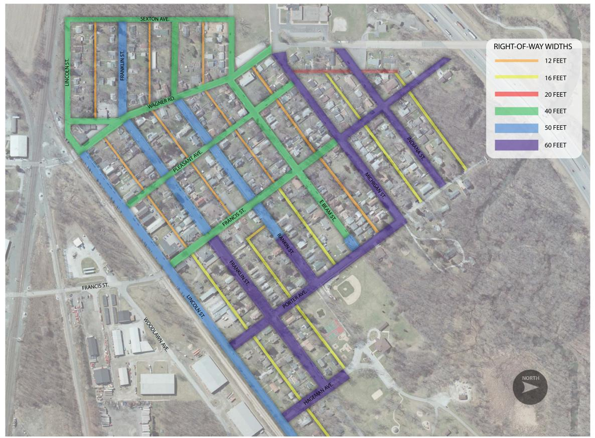
Figure 2-1. Right-of-Way Widths.
