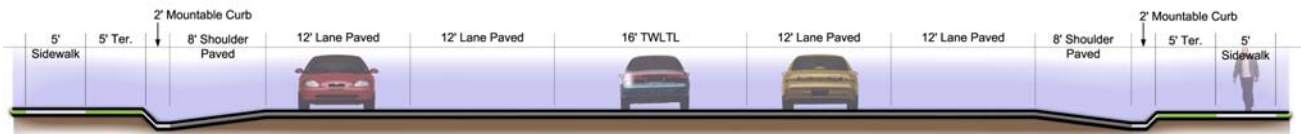
Figure 13 – Five-Lane with Two-Way Left Turn Lane Cross-Section
