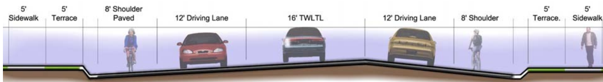
Figure 17 – Three-Lane with Two-Way Left-Turn Lane
