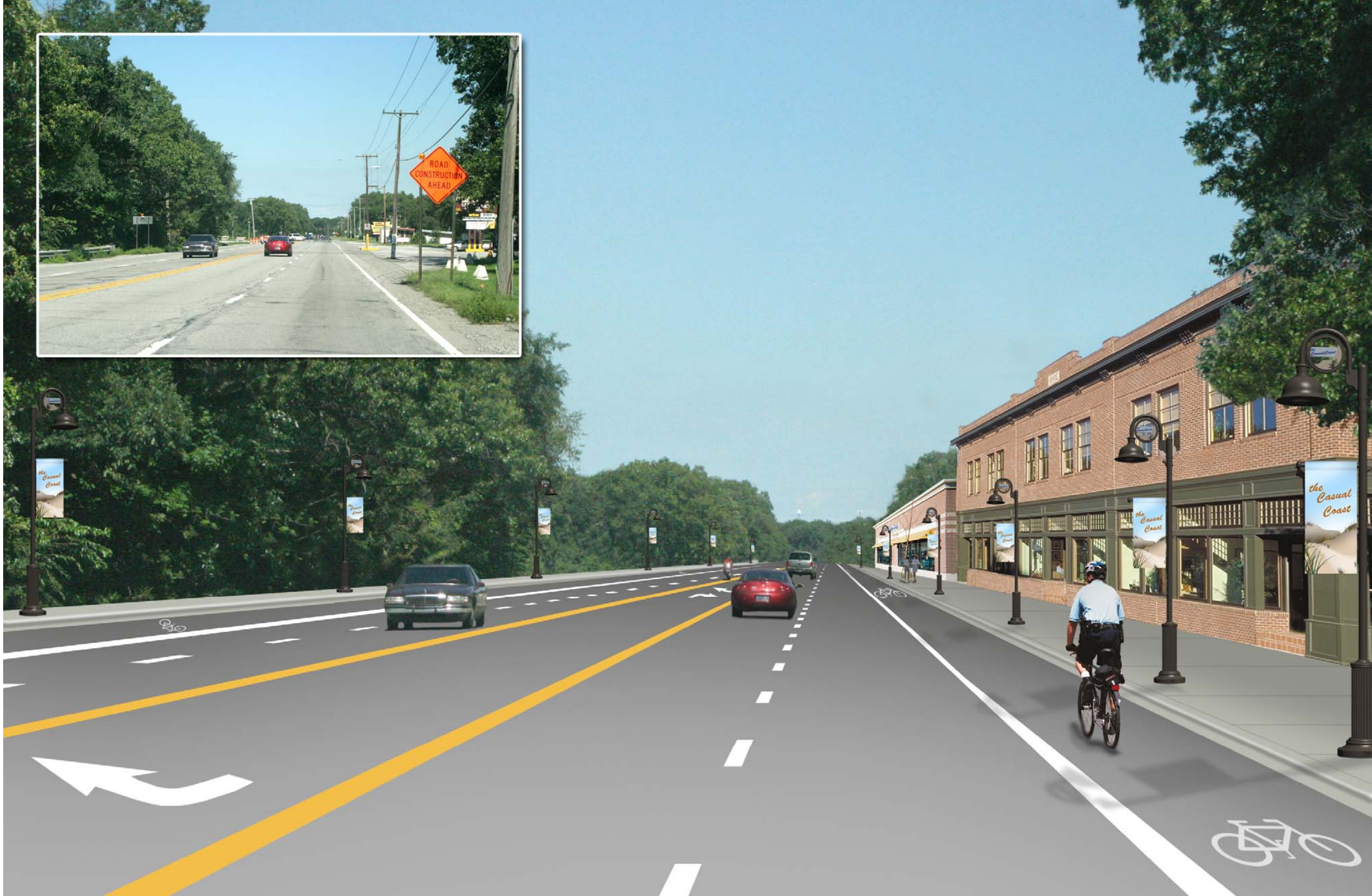
Figure 14 – US-20 Five-Lane with Two-Way Left Turn Lane
