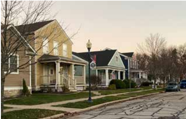
Village at Burns Harbor (small lot single-family): Net density – 9 du/acre; gross density – 7.6 du/A
