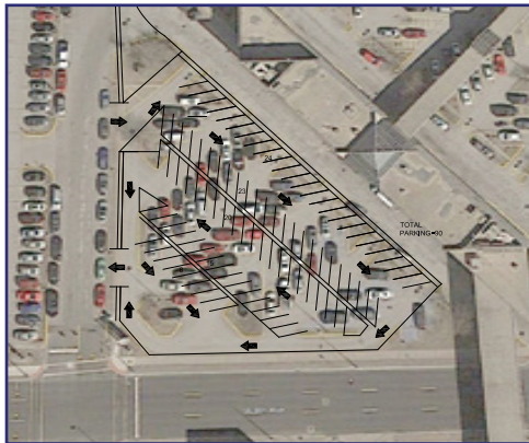
THIS CONCEPT FOR ADAM BENJAMIN CENTER PARKING RECONFIGURATION IMPROVES TRAFFIC FLOW WHILE ADDING OVER 20 SPACES TO CURRENT LOT
