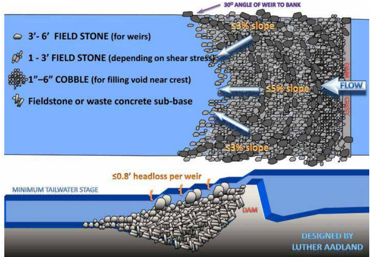
FIGURE 6.1-2 | Typical Rock Riffle Structure
