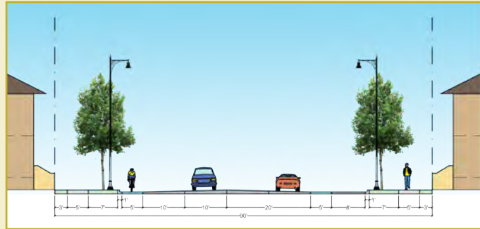
CONCEPT- COMPLETE STREET, MAINTAIN PARKWAY; MEDIANS WHERE NO TURN LANES NEEDED, NO PARKWAY SOUTH OF ALLEY
