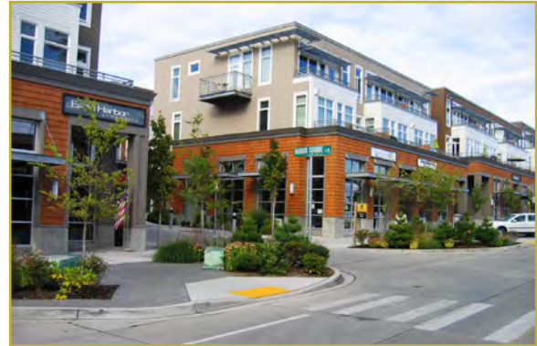
THIS CURB EXTENSION HELPS TO CALM TRAFFIC AND ALLOWS FOR INCREASED LANDSCAPING AND PUBLIC PLAZA SPACE
