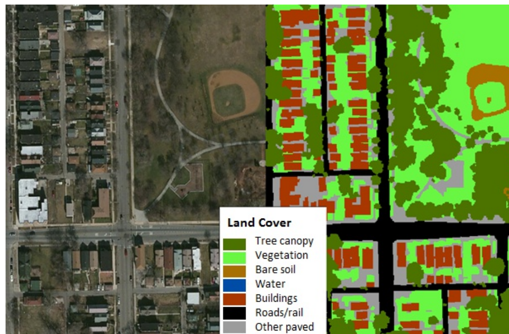
Fig. 1: Comparison of satellite image and land cover map. Seven types of gray and green infrastructure are in the land cover map.
