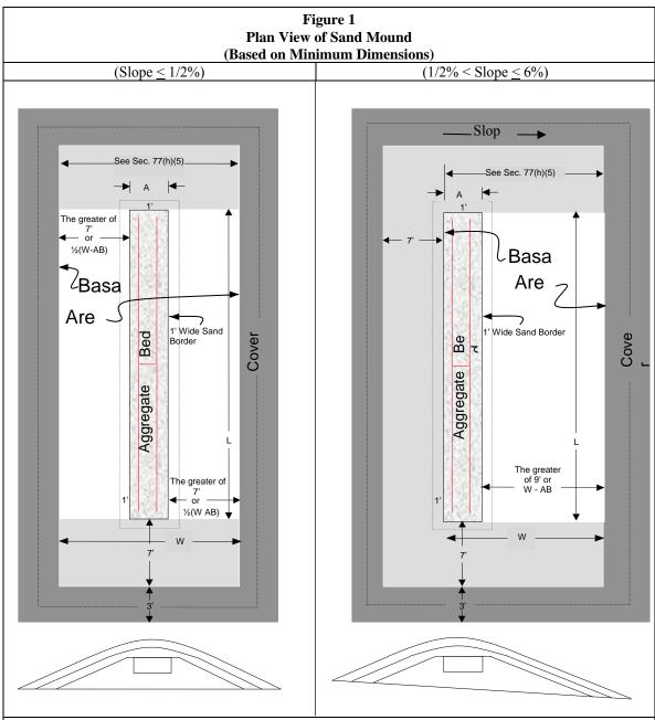
Legend: L = length of aggregate bed; AB = width of aggregate bed; W = total width of basal area. Schematic is for a 12" sand depth below the aggregate bed, and an aggregate bed depth of 6" below the laterals, plus the diameter of the laterals, plus 2" above the laterals.
