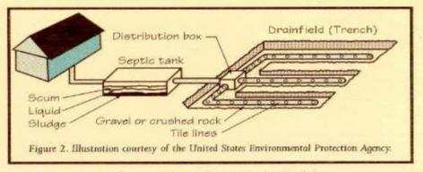
Schematic of a Drainfield
