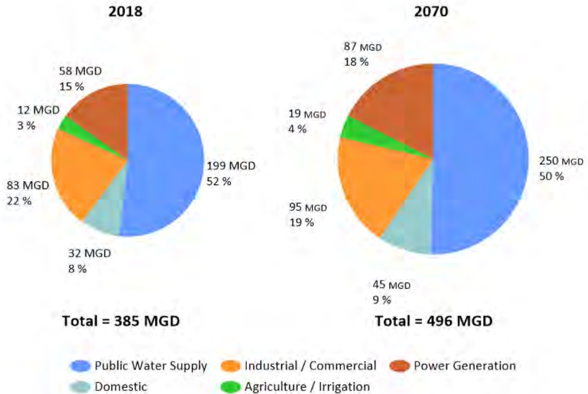
Figure A: Regional water withdrawals by water-use sector for the Central Region in 2018 and forecasted withdrawals for 2070. Regional annual average withdrawals are expected to increase 111 MGD from 385 MGD in 2018 to 496 MGD in 2070. All sectors are expected to increase. Public water supply comprises ~50% of the total throughout the forecast. Annual 2018 historical water withdrawals are from the Indiana Department of Natural Resources Significant Water Withdrawals Database, 1985-2018 (DNR, 2018). Central Region includes the following nine counties: Boone, Hendricks, Hamilton, Hancock, Johnson, Madison, Marion, Morgan, and Shelby.
