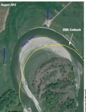
Where coal ash disposal sites are adjacent to rivers, as is the case at Gibson and Cayuga, channel migration could erode into the coal ash disposal structures over time causing release of the ash. This will be particularly true after Duke's maintenance obligation ends.
