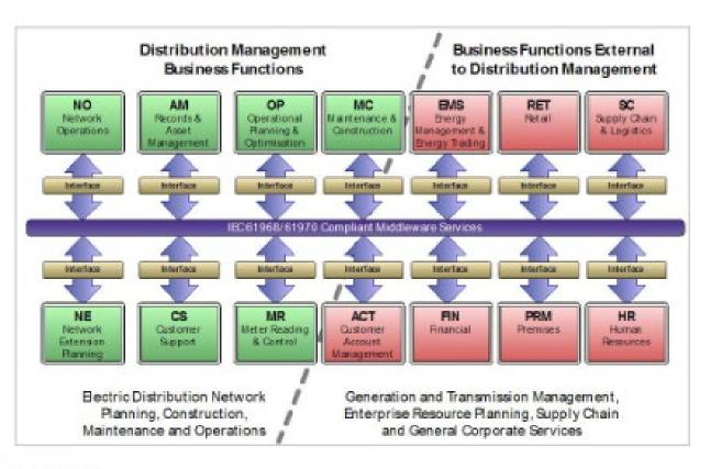
Figure 6-1 IFC61968-1 Interface Reference Model
