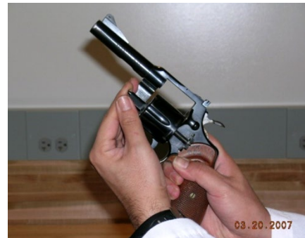
Step 2: Eject any cartridges from chambers
