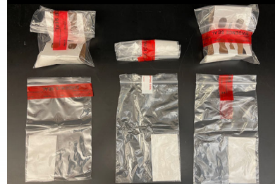
Improperly Sealed Secondary Containers
