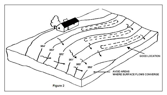
The area for the proposed absorption field and immediately down slope from the absorption field area must be protected from traffic and construction to avoid disturbing the area. Construction and traffic in this area can cause the soil to become compacted and result in failure of the system. It is recommended that this area be fenced (construction fence) off to assure adequate protection.
