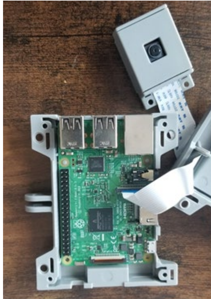
Figure 1. Affordable technologies for measuring crop growth and plant nitrogen status being developed by Principal Investigator at Purdue University. a. Microcontroller interfaced to a camera, b. smartphone-based sensing
