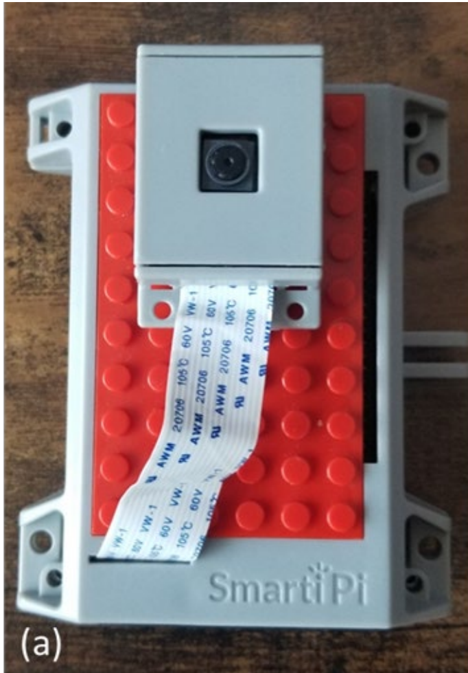
Figure 1. Affordable technologies for measuring crop growth and plant nitrogen status being developed by Principal Investigator at Purdue University. a. Microcontroller interfaced to a camera, b. smartphone-based sensing
