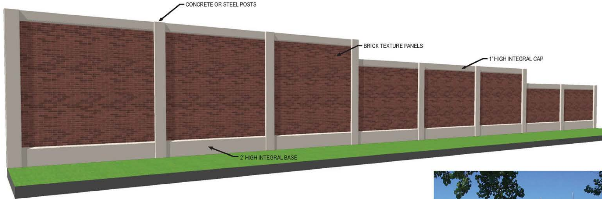
▲ Brick texture sound wall
