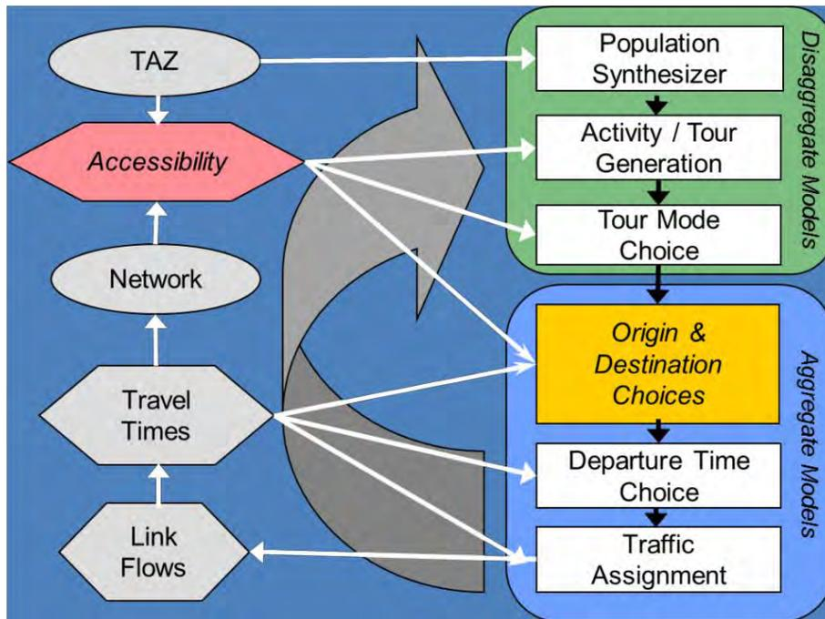
The corridor model utilizes outputs from the Indiana Statewide Travel Demand Model Version 7 (ISTDM v7) to identify the pattern of trips originating or ending outside of the four-county study area. The corridor model then determines the optimal route of these trips through the study area.
