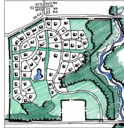
Cluster Zoning example illustrating the removal of the existing farmstead, a larger buffer for the natural stream corridor, and small greenways traversing the community. This option allows for added connectivity, shared greenspace, and greater protection of natural features.
