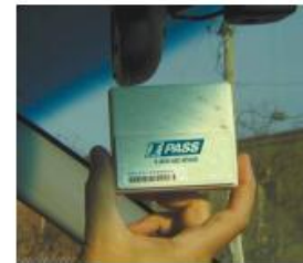
Transponder attaches to windshield
