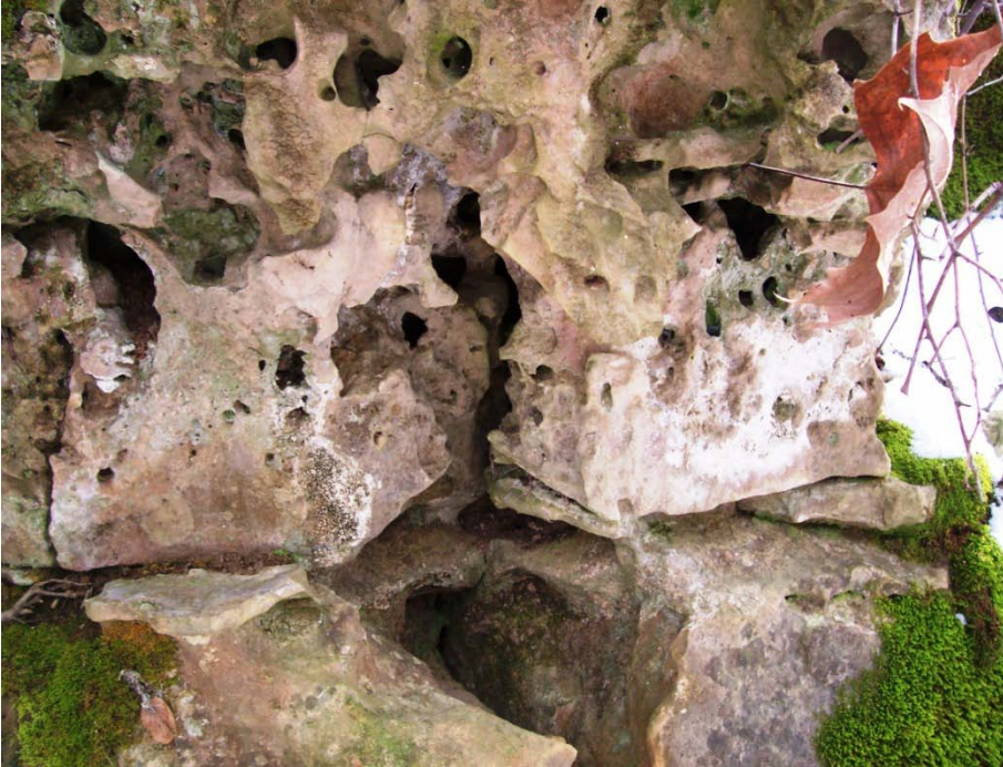
Photo 145: General, Typical exposed bedrock of the area – limestone with large volume of vugs and fractures.
