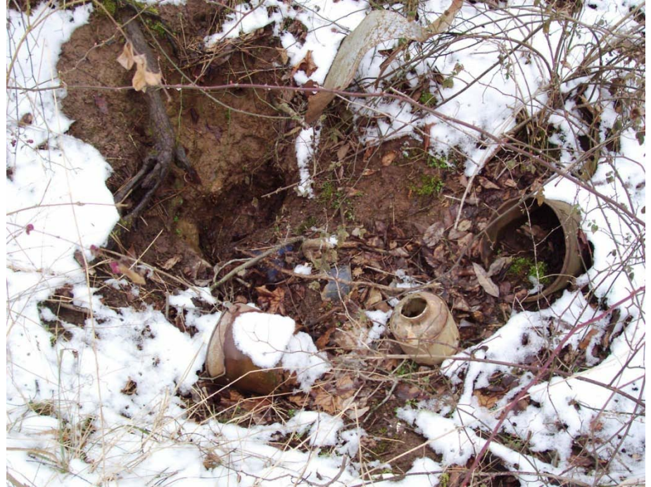
Photo 120: E-18, E-19 & E-20, Swallow hole with debris in one of a cluster of sinkholes with multiple large swallow holes.
