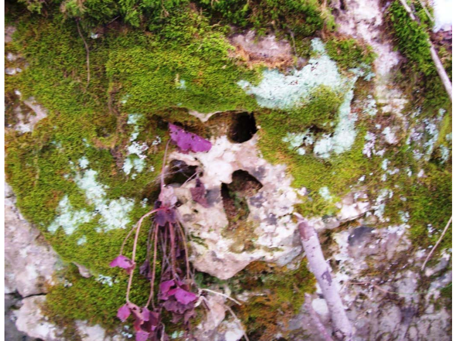
Photo 144: General, Typical exposed bedrock of the area – limestone with large volume of vugs and fractures.
