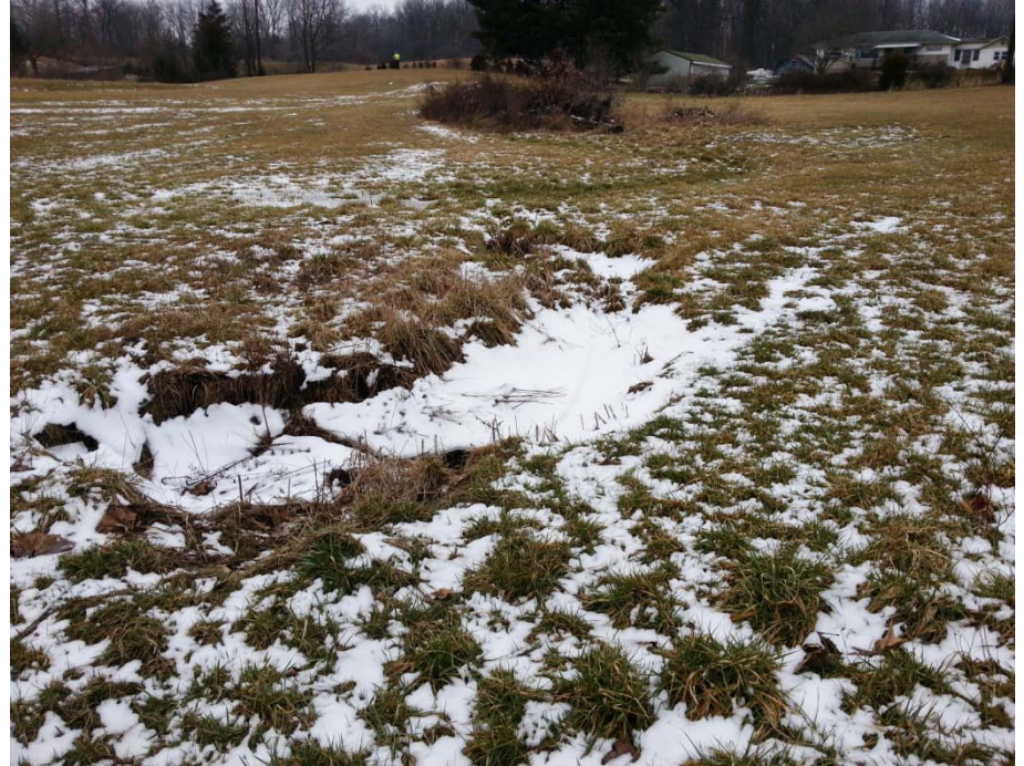
Photo 18: A-08, Line of small depressions, approximately 20' long x 5' wide x 2' deep, snow covered.
