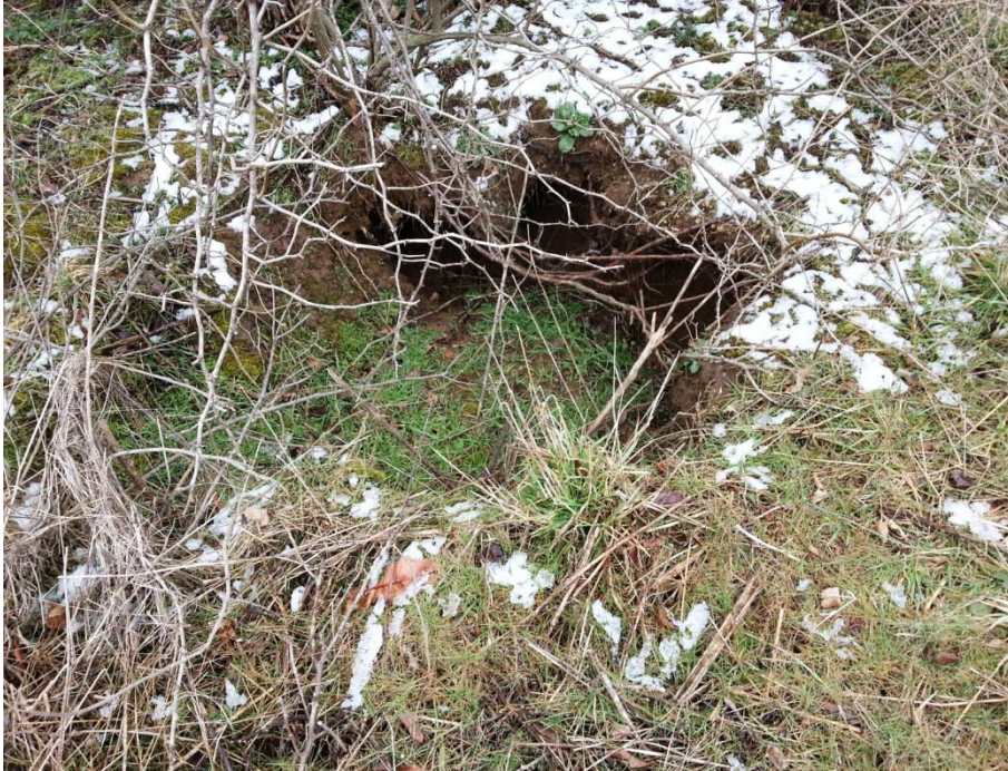
Photo 41: C-03 & C-T2, Swallow hole within a large broad silt filled sinkhole with several distinct 2' diameter x 2' deep swallow holes approx 80 long x 40' wide with 5' total depth.
