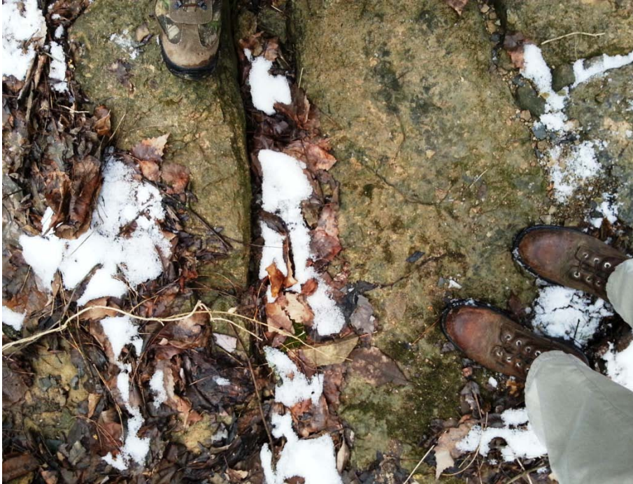
Photo 1: A-01, Joints in creek bed at 160-170 degrees with a secondary joint at 80 degrees
