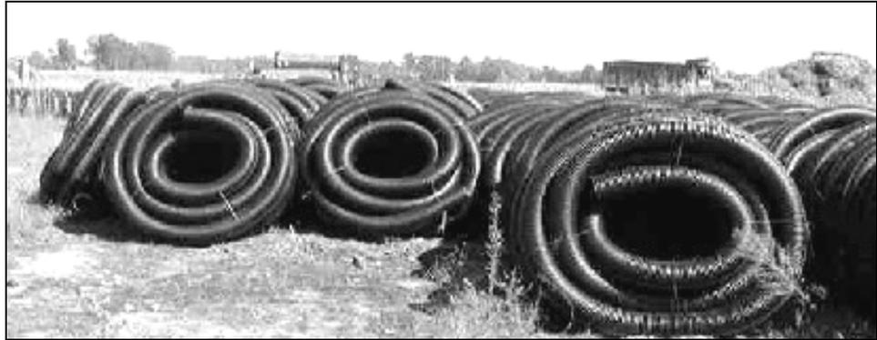
**Figure 10-1. Plastic Corrugated Drainage Pipe**
