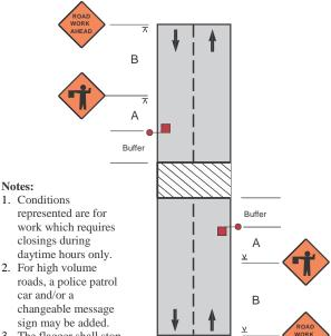
3. The flagger shall stop the first vehicle from the shoulder as shown. After stopping the first vehicle if the view of the flagger is obstructed, then he/she should move to the centerline to stop additional traffic.
