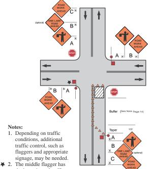
the best view of traffic from all directions. This flagger should be designated lead flagger and should coordinate the actions of the other flaggers.
