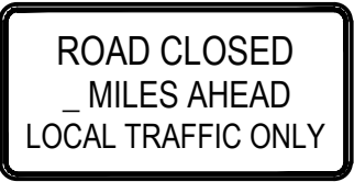
ROAD CLOSURE SIGN ASSEMBLY - TYPE 1
