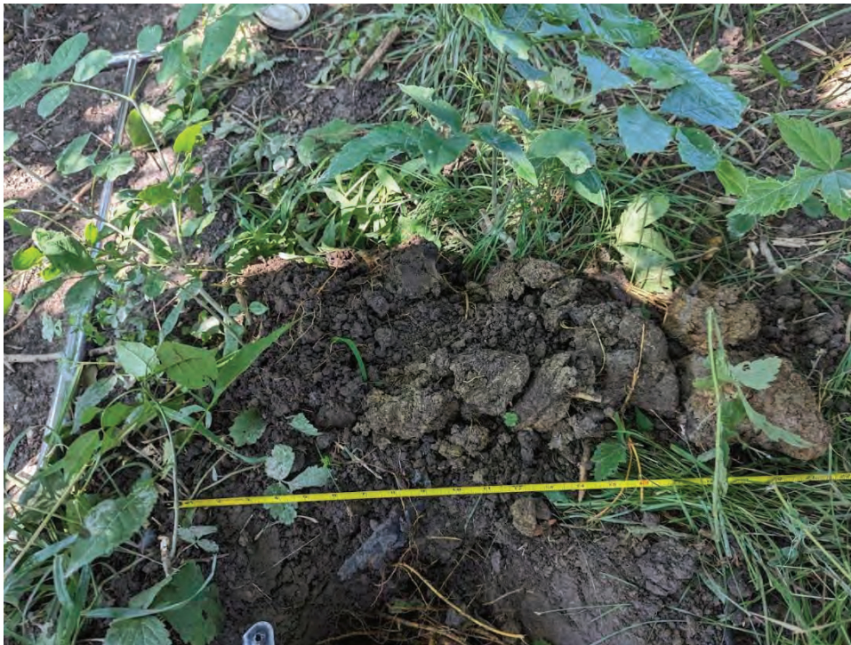
Photograph 38. View of the soil profile of SP4 which met the Depleted Below Dark Surface (A11) and Depleted Matrix (F3) hydric soil indicators.
