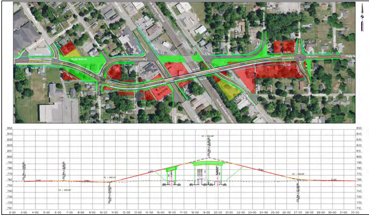
Figure 1-2 Alternate 3A Realign Hively to South (Connection Roadway to North) - Plan & Profile
