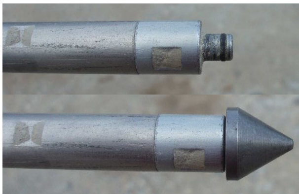
Figure 13-2 No Tip Installed (Top) Disposable Tip (Bottom)
