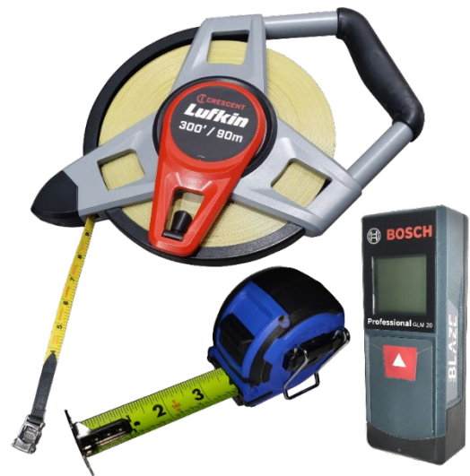
Figure 3-4 Cloth, Pocket, and Laser Tapes
