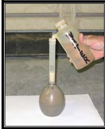
Figure 7 Adding Water to Calibrated Capacity
