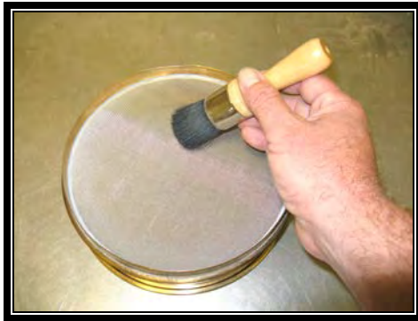
Figure 4 Use Hair Brush on Fine Sieves
