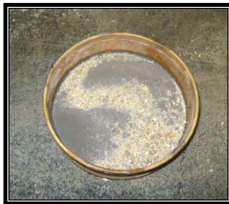
Figure 4 Material Retained on the No. 200 (75 \mu\text{m} ) sieve
