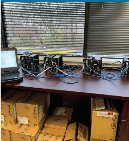
Bench testing of network switches prior to installation on the gantry
