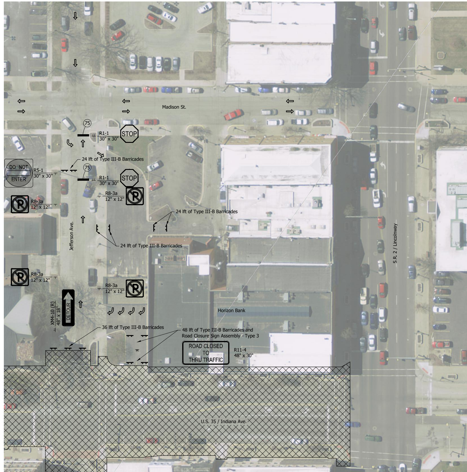
HORIZON BANK TEMPORARY MAINTENANCE OF TRAFFIC Scale: 1" = 30'
