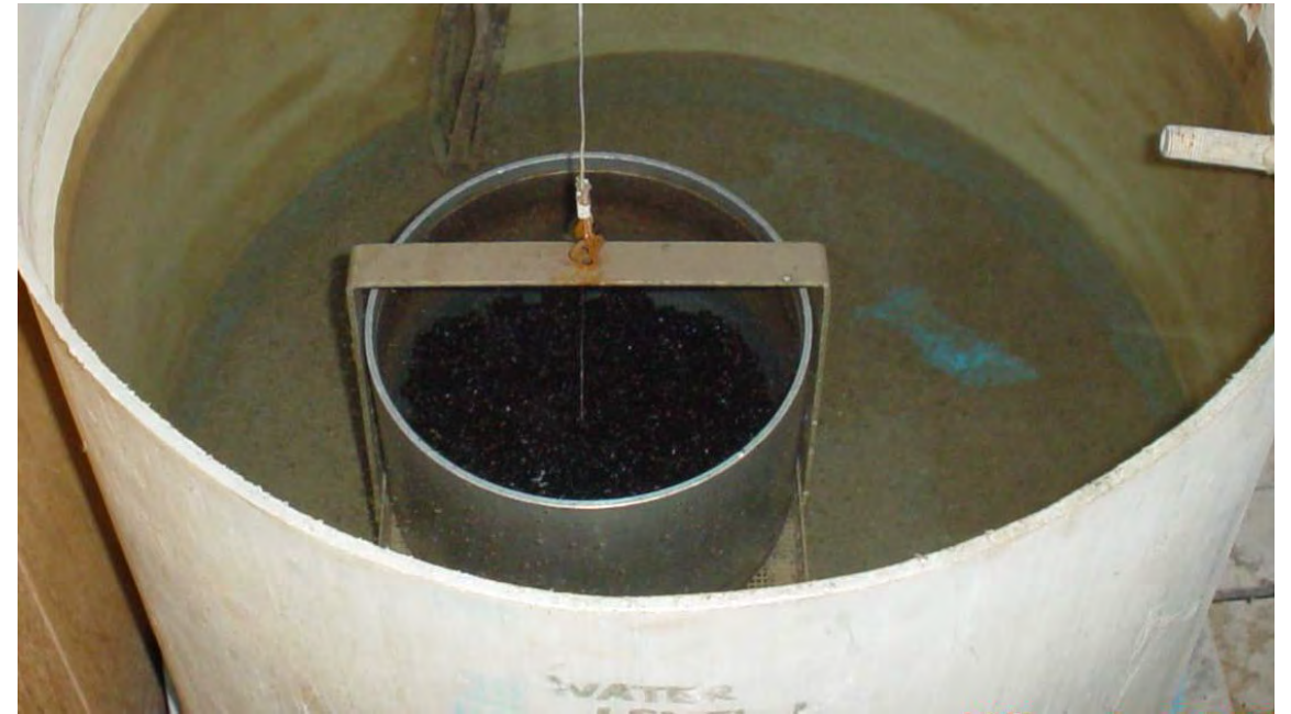
Bowl and Sample weight under water
