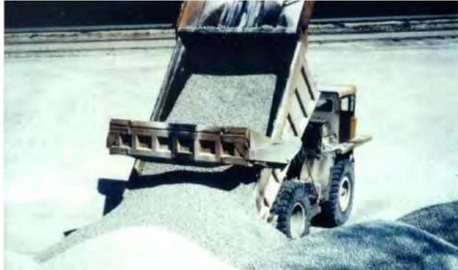
Figure 4.28 Truck Built Stockpiles
