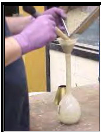
Figure 5 Pouring sand into pycnometer once SSD is achieved
