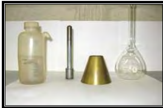
Figure 1 Fine Aggregate Specific Gravity Apparatus
