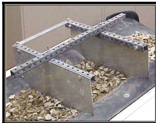
Figure 2 Conveyor Belt Sampling
