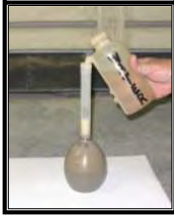
Figure 7 Adding Water to Calibrated Capacity
