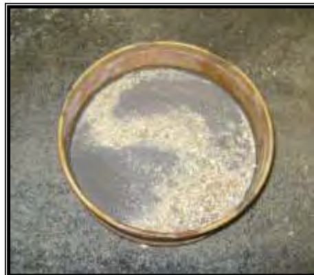
Figure 4 Material Retained on the No. 200 (75 \mu m) sieve
