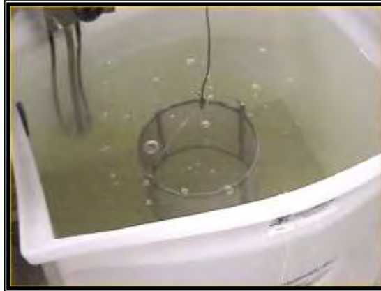
Figure 1 Coarse Aggregate Gravity Apparatus
