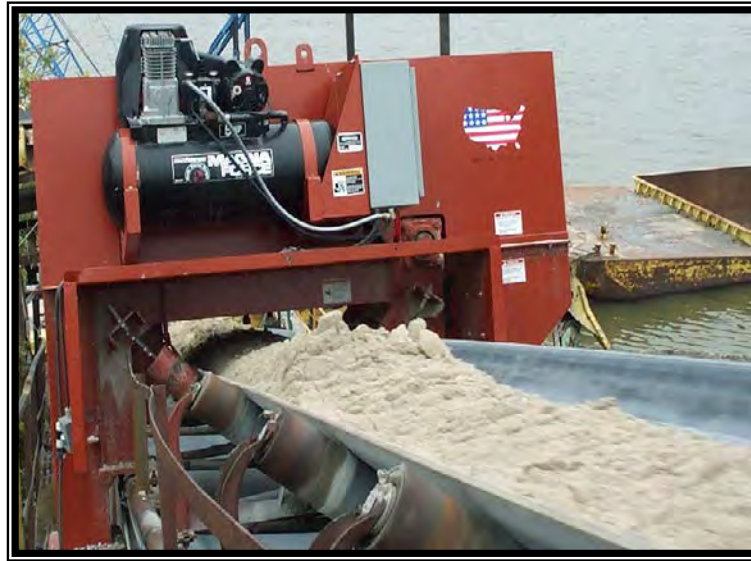
Figure 3 Automatic Sampling Device
