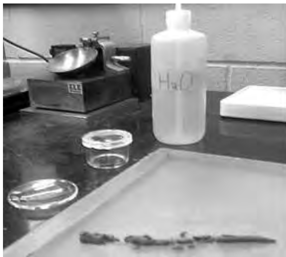
Figure 8.17 Field Check Plastic Limit Test
