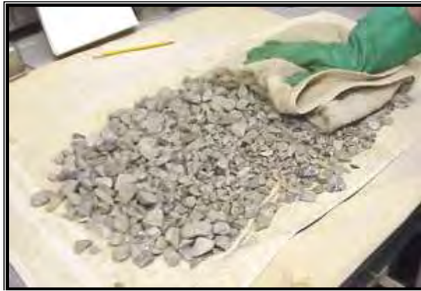
Figure 8 Removing Excess Water
