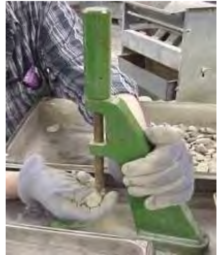
Figure 8.13 Scratch Hardness Test
