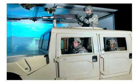
RVTT - Reconfigurable Vehicle Tactical Trainer provides four simulated vehicles in a 360 degree virtual environment
