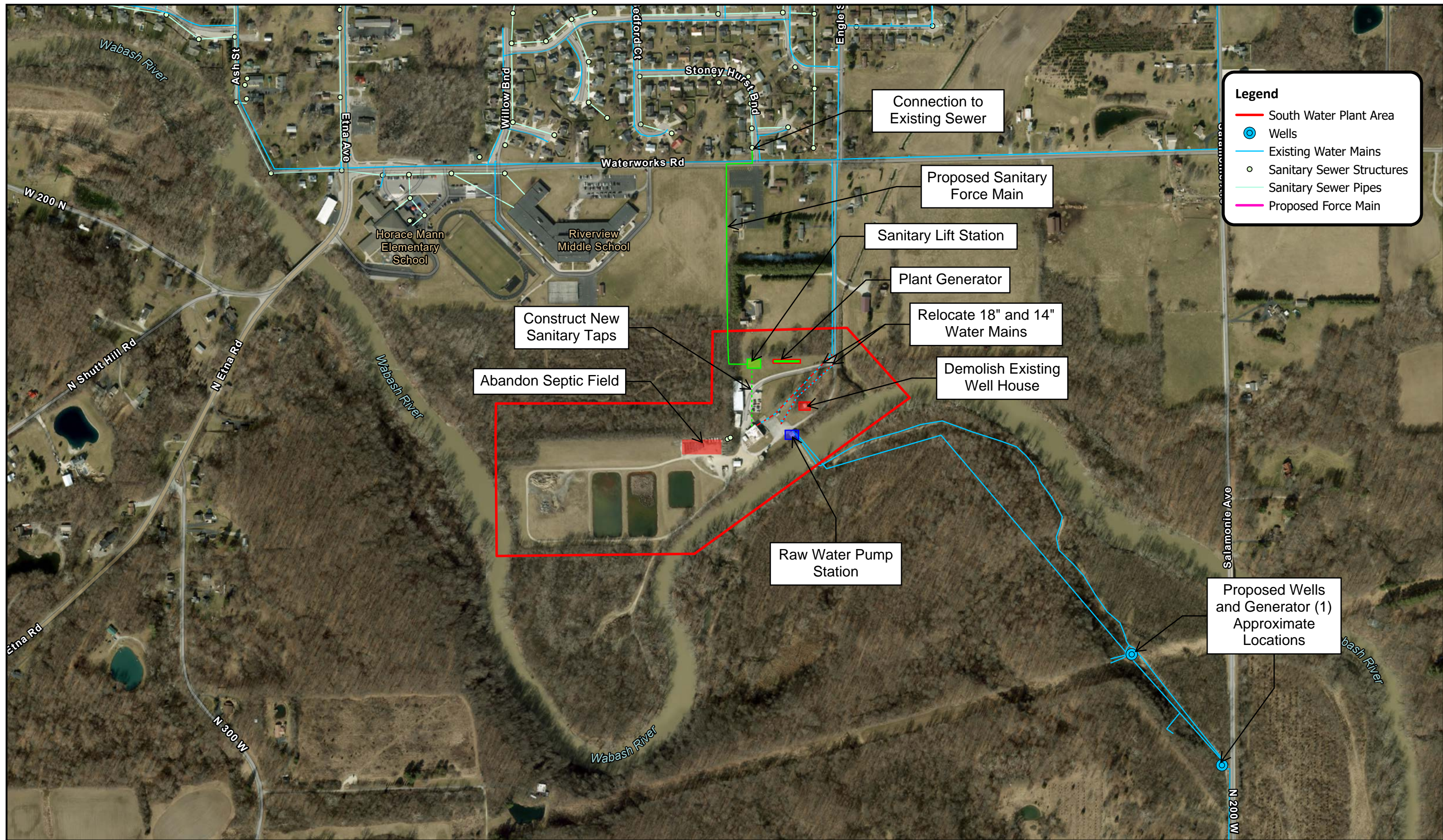
Figure 1 - Phase 1 South Water Treatment Plant Replacement Project Huntington, Indiana
