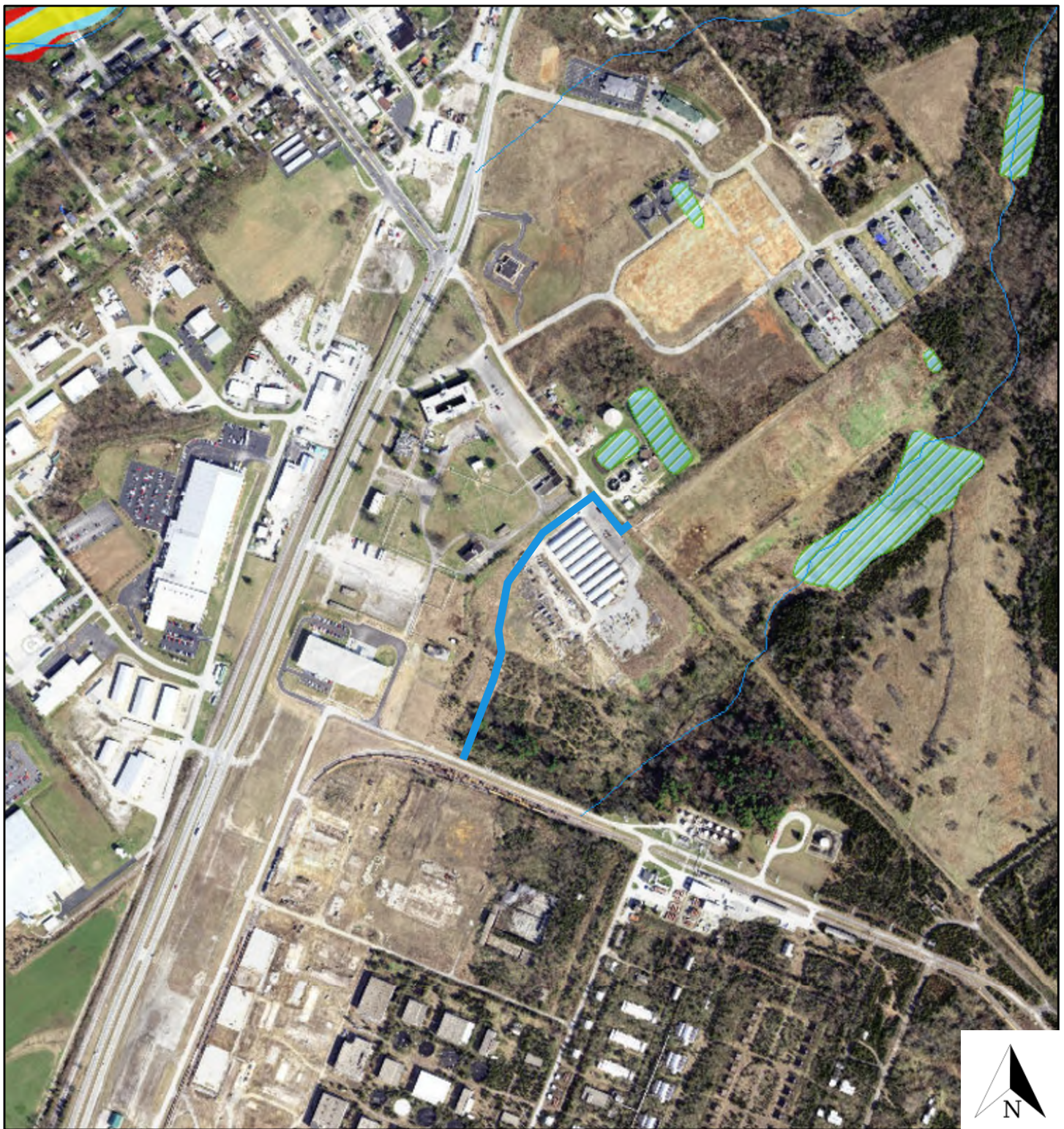
Figure 5b: Water Main Connection to RRDA Wetlands/Floodplains
