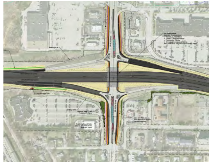
Figure 4.2-24: SR 48/3rd Street Intersection Enhancements
