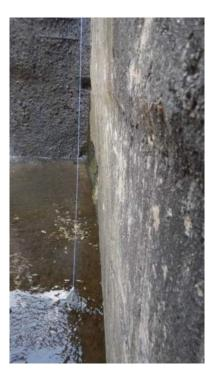
**Photo A11:** View of a measurement of the RT spillway abutment wall tilt.
