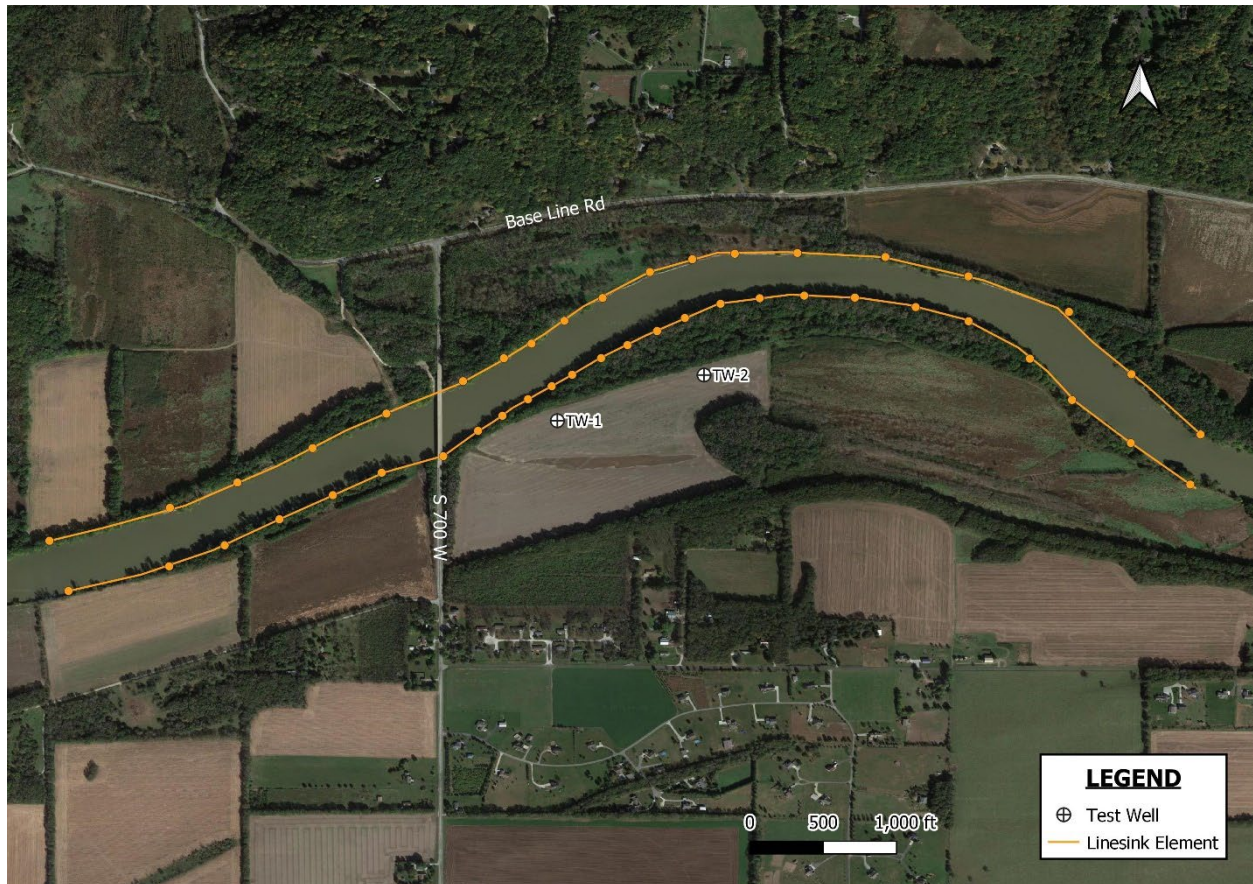
Figure 8. Layout of analytic elements used in TTim modeling analysis.
