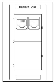
3.9 Single Mode Fiber PIC Faceplate Configuration in a Single-Gang Faceplate:
