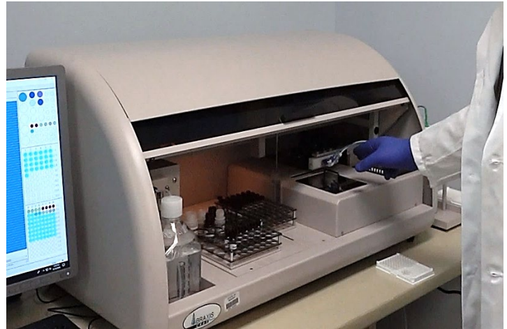
IDEM staff use the cyanotoxin automated assay system (CAAS) equipment to analyze microcystin, cylindrospermopsin, anatoxin-a, and saxitoxin in beach water samples.
